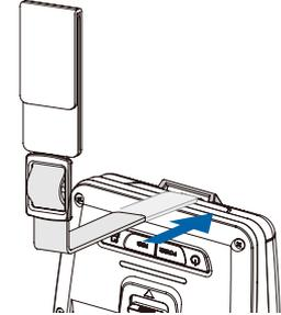
Put the strap into the strap bracket hole as shown.
