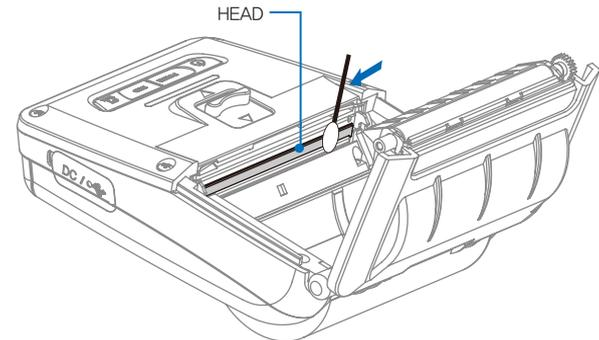
1. Use an applicator swab moistened with an alcohol solution to clean the printhead and remove any dust.
