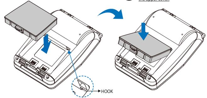
1. Align battery hook as shown in the picture.
