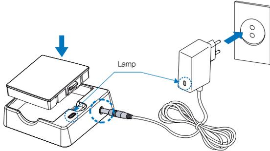
1. Insert the battery into the battery charger as shown above.
