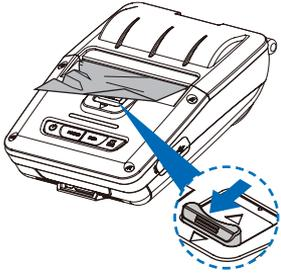
When you face with a paper jam error, please press the button down to open the printer cover.
