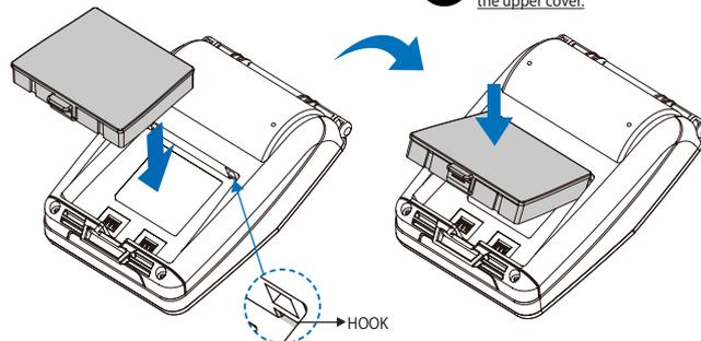
1. Align battery hook as shown in the picture.
