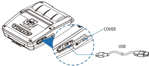
1. Flip over the connector cover and connect USB cable to the printer connector.
