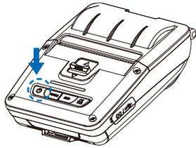
Turn off the power by pressing the power button for approximately 3 seconds.
