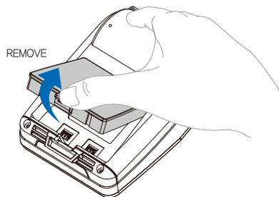
Remove the battery as shown.
