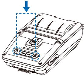
While you are holding the FEED button, press the power button.
